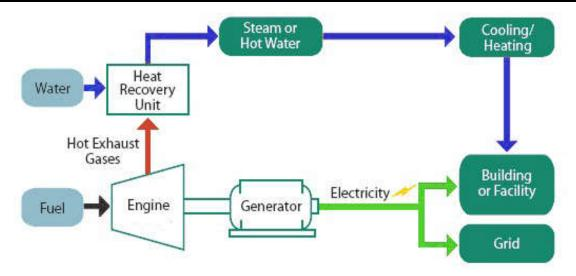
We offer Combined Cooling Heating and Power (CHP and CCHP) packages for our gas generator sets. It can recover 75%-90% combined electrical and thermal efficiency, resulting in major reductions in your overall energy costs. In the past years we have supplied CHP systems to Germany, Russia,Indonesia etc. We have the experience and capabilities to meet your total energy requirements.
