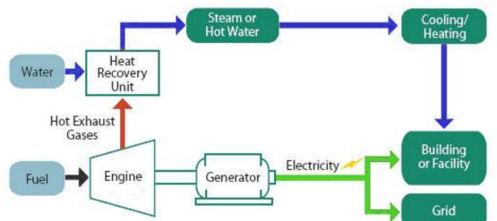
We offer Combined Cooling Heating and Power (CHP and CCHP) packages for our gas generator sets. It can recover 75%-90% combined electrical and thermal efficiency, resulting in major reductions in your overall energy costs. In the past years we have supplied CHP systems to Germany, Russia, Indonesia etc. We have the experience and capabilities to meet your total energy requirements.
